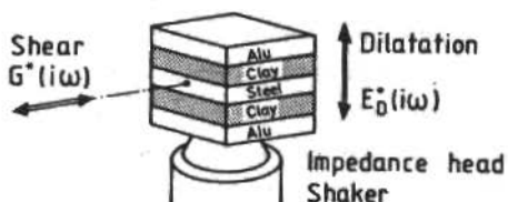
Figure 8. Clay sandwich for alternating dilatation and shear tests
