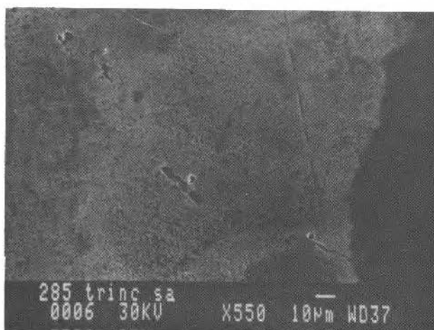
Fig. 7 Hydrogen Induced Cracking in ASTM 285 Grade G Sample (550x)
