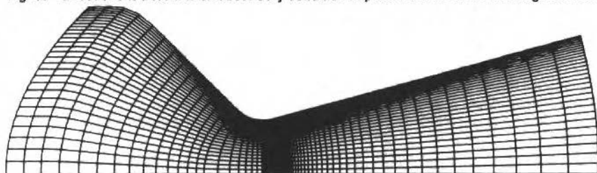
Fig. 19 Computational mesh and nozzle geometry for realistic axisymmetric nozzle computations.
